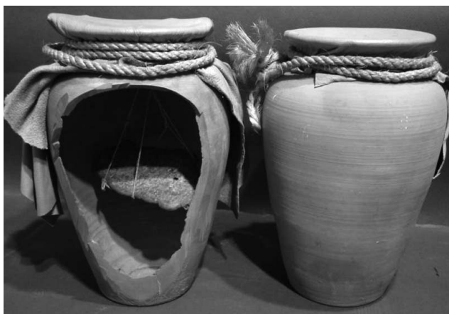
Figure 8: Reconstruction of the apparatus according to Theophrastus in his text "On Stones" for the preparation of the psimythion (lead white).
