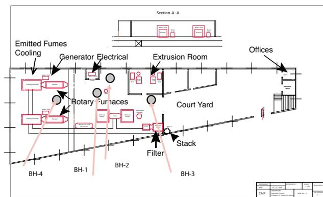
Figure 3. Borehole well location map (BH-1 through BH-4)
