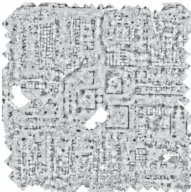
Figure 4: GPR depth slice 0.20-0.40 m. A Wallis-Filter with a 12 x 12 m window enhances archaeological structures with very small geophysical contrast.
